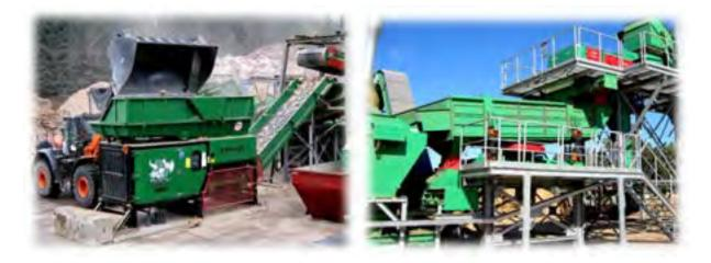
The value of the wood will be upgraded with a HAAS wood grinder, consisting of pre - and after shredding. The operation includes ferrous and non-ferrous separation, with a throughput of 20 tons per hour. Oscillating screens can vary the chip size with easy and uncomplicated screen changes.
