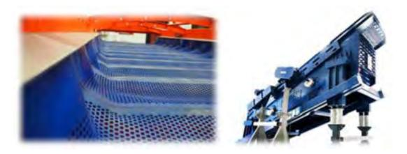
The 0-2" material is split again by a flip flow fines screen with hole spacing sized to remove  $\frac{1}{2}$ " minus material, or fines. A very large percentage of the fines fall through the holes and are conveyed out to a central load out area. These fines could then potentially be used as alternate daily landfill cover (ADC). The newly created  $\frac{1}{2}$ "-2" fraction is conveyed to a Two Way Walair separation unit.
