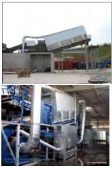
The WAL-AIR Drum Air Separator is a highly versatile piece of equipment with multiple variables that can be adjusted to pinpoint specific separation of MSW based on weight and density. This two way WAL-AIR device separates the MSW into two different density streams: "heavies" and "lights".
