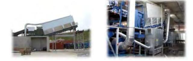
The WAL-AIR Drum Air Separator is a highly versatile piece of equipment with multiple variables that can be adjusted to pinpoint specific separation of C&D material based on weight and density. This two way WAL-AIR device separates the material into three different density streams: "heavies" and "lights".
