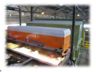
would be conveyed to residue compactors. The high resolution and precision accuracy of the TOMRA ejection systems provides very high recovery of clean wood.
