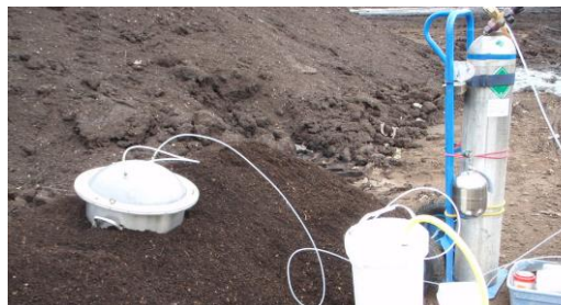
Photo 3.4 USEPA Flux Chamber
