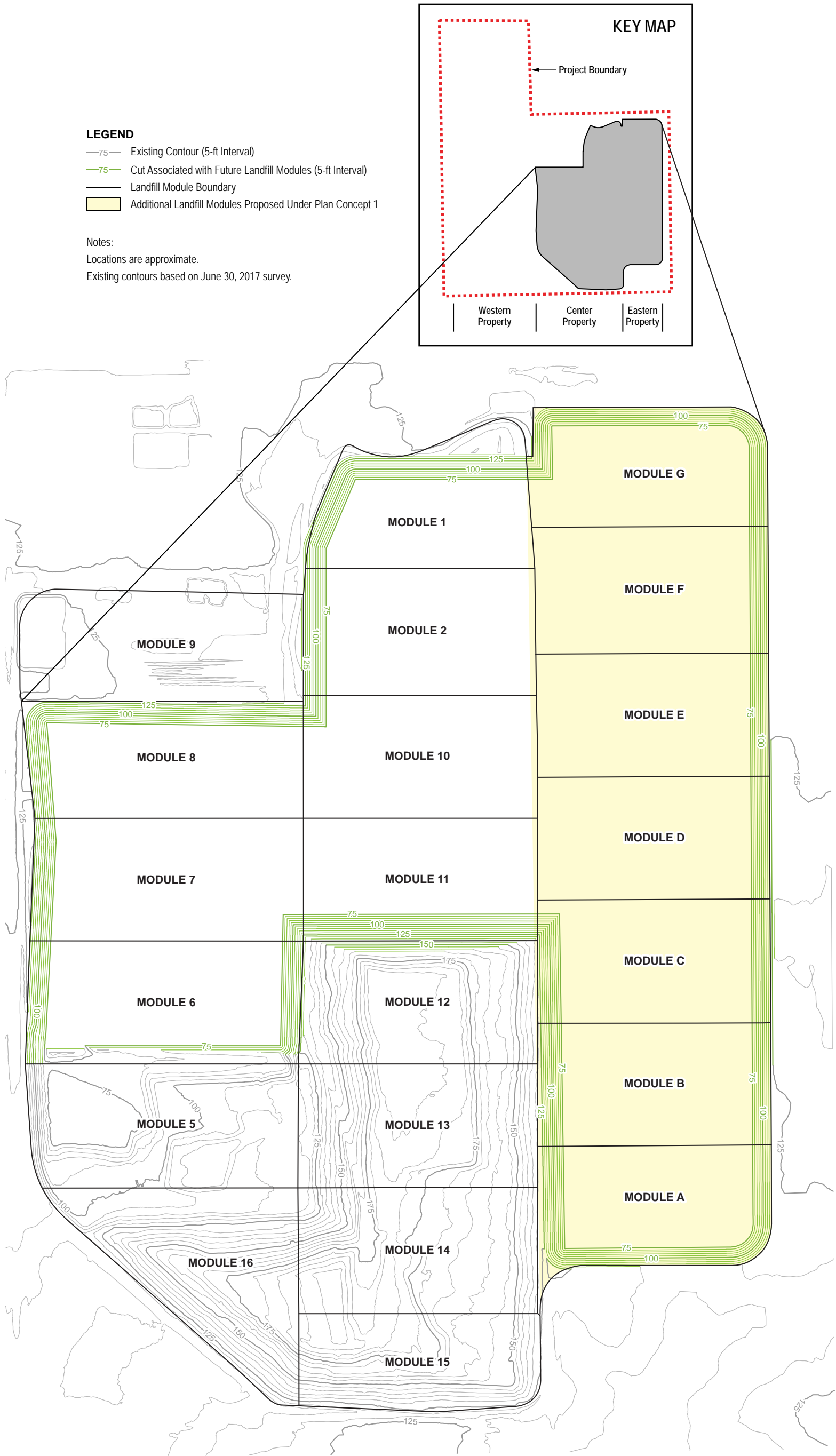
Figure 3-3. Plan Concept 1 WRS� Anticipated Fill Sequence Draft Environmental Impact Report Renewable Placer: Waste Action Plan Placer County, California
