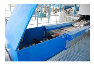
The single Eddy Current per line is for the recovery of aluminum (AL) and some other NF. AL is propelled over the eddy current's adjustable gate and is then air conveyed to a storage bunker for baling.
