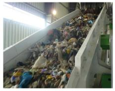
SPALECK is a leader in screening technology. The 3D Waste screen does very accurate sizing in three dimensions while providing almost blockage-free screening, minimum effort for cleaning with very good accessibility, and very low operating costs due to maximum machine availability.
