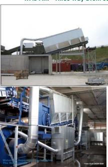
The WAL-AIR Drum Air Separator is a highly versatile piece of equipment with multiple variables that can be adjusted to pinpoint specific separation of MSW based on weight and density. This two way WAL-AIR device separates the MSW into two different density streams: "heavies" and "lights".
