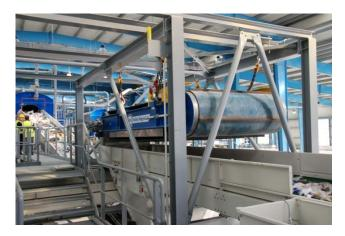
There are five Cross Belt Magnets in the sorting system. All magnets are sized accordingly to recover the FE metals of various sizes and densities from the different stages throughout the system. Based on VDRS experience, we realize that simply having one magnet to capture all FE metals is not possible – our design has three magnets per line, positioned in the proper locations.
