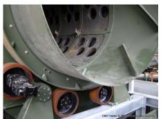
The 3D Trommel Screen has openings to separate MSW material that is less than 16"
